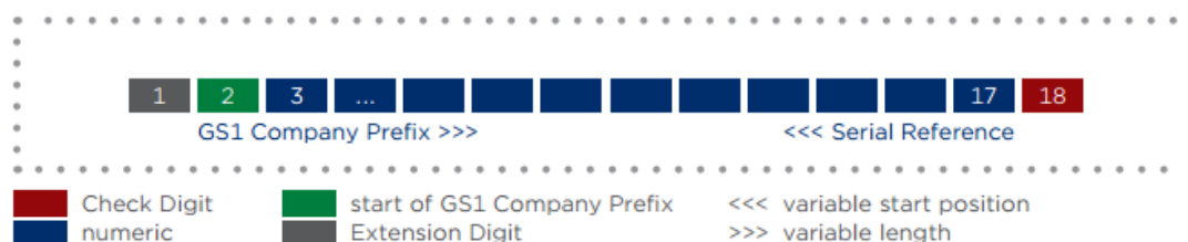
Figure 8-1 SSCC Data Structure
